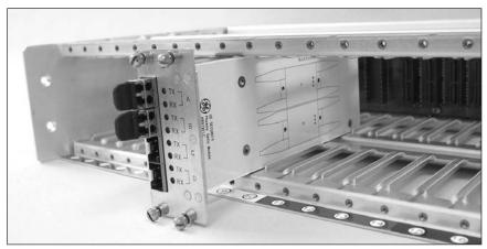
**INSERT OPTICAL TRANSCEIVER MODULES IN SLOTS 9-10 (White)**
